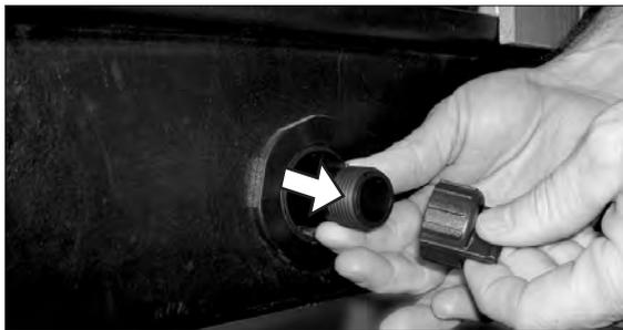
**Step 5:** Attach a standard garden hose. Push the drain spout in halfway to actuate the drain.
