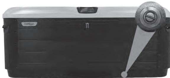
**Step 3:** Pull the drain out with a slight clockwise turn. Use pliers if needed.
