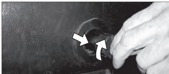
**Step 4:** Remove drain cap.
