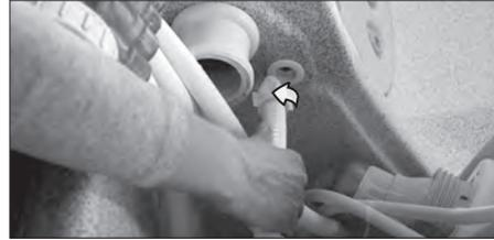
**Step 5:** Disconnect the air line union and remove the JetPak from the JetPod.
