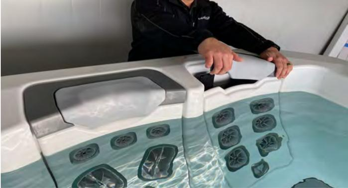
**Step 3:** While applying pressure downward on the manifold push the manifold toward the inside of the spa to release the manifold from the wall clip assembly, then lift the jet plate straight up to remove.
