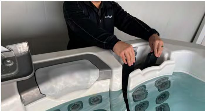
**CAUTION!** WHILE PERFORMING STEPS 3 AND 4 YOU MUST USE THE BLACK MANIFOLD AREA AS THE POINT OF CONTACT AS SHOWN IN THE PICTURE. PRESSURE APPLIED TO THE FRONT FACE (ACRYLIC PLATE) MAY CAUSE DAMAGE TO THE JETPAK VOIDING THE WARRANTY
